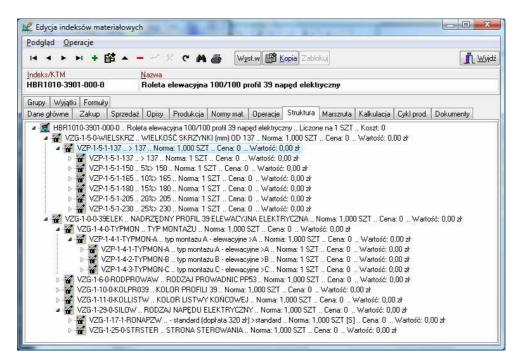
Fig. 5. Implementation of "AND/OR graph" in PDM module for roller shutter
