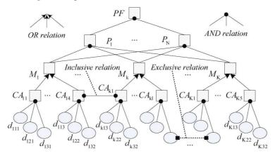
Fig. 4. AND/OR graph representation of configuration space [24]
